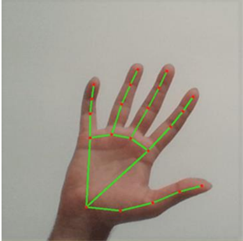
Fig. 2. MediaPipe system working with Hand tracking
