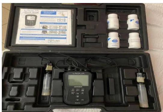
Plate 1: Showing Photograph of Horiba PC210 water meter
