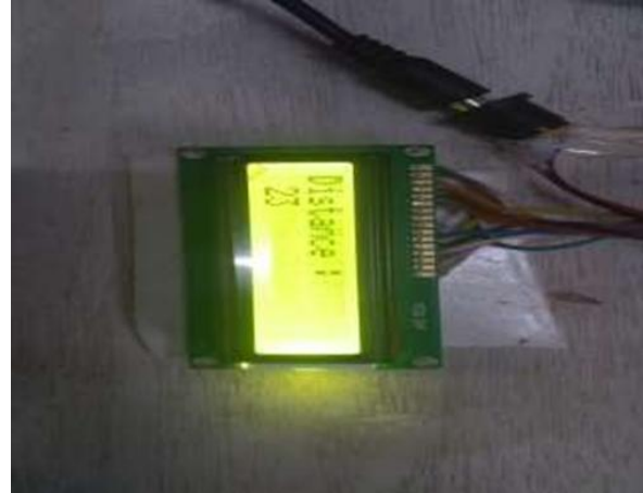
Fig. 10. Displaying distance of the train from the Railway gate
