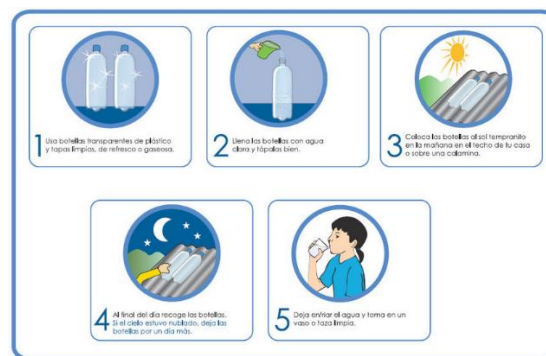
Figure 2: Five-step protocol for handling the SODIS method (Hobbins, 2006).
