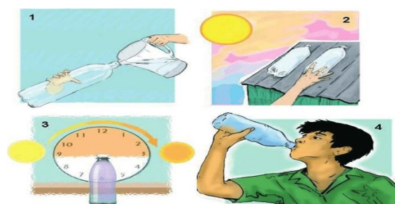
Figure 4: A graphical description of the solar disinfection (SODIS) technique (Keane, et al., 2014).
