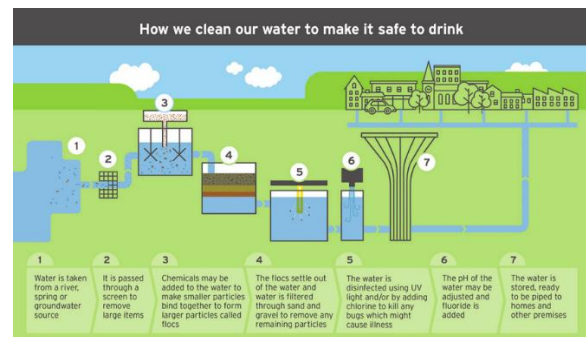
Figure 2: Drinking water treatment (Treacy, 2019).
