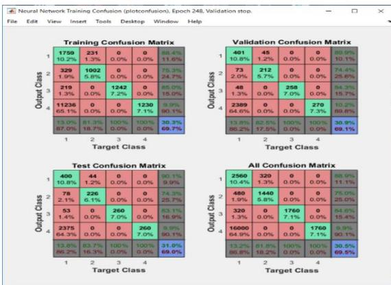
Figure 4.21: Confusion matrix for ANN locating faults on lines of section 1 of Zone 1
