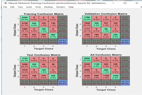
Figure 4.31: Confusion matrix for ANN locating faults on lines of section 1 of Zone 2
