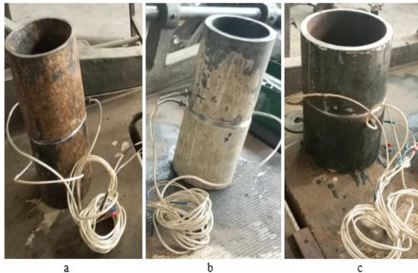
Figure 1.1: Steel oil pipe connected with three K-type thermocouples positioned 10 mm, 12 mm, and 15 mm away from the weld centreline before the welding operation. (a) 90 mm diameter by 5 mm thick pipe, (b) 100 mm diameter by 10 mm thick pipe, and (c) 140 mm diameter by 15 mm thick pipe.
