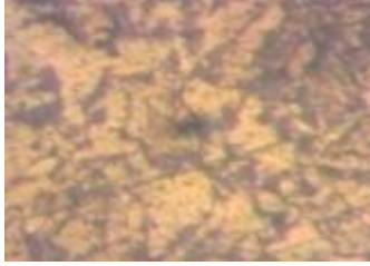
Plate 6: Microstructural analysis of LCS HAZ hardened in Groundnut oil Quenched steel.
