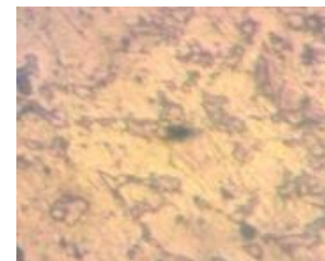
Plate 4: Microstructural analysis of LCS HAZ hardened in Palm oil.
