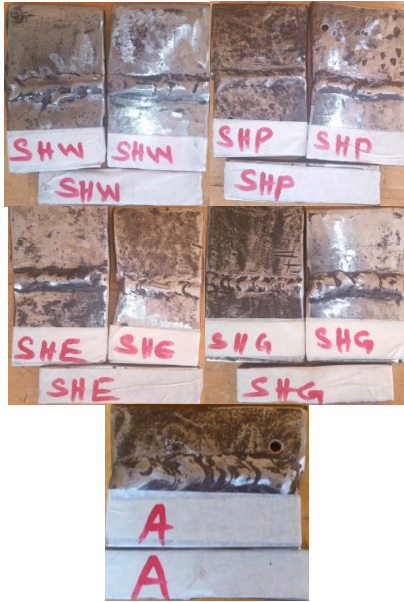
Plate 1: Experimental procedure shows an array of the specimen after SMAW welding operation.
