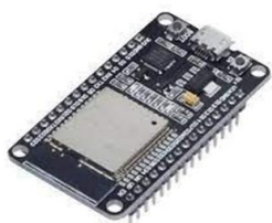
Figure 1: ESP32 Development Board WIFI+BT W/ Antenna
