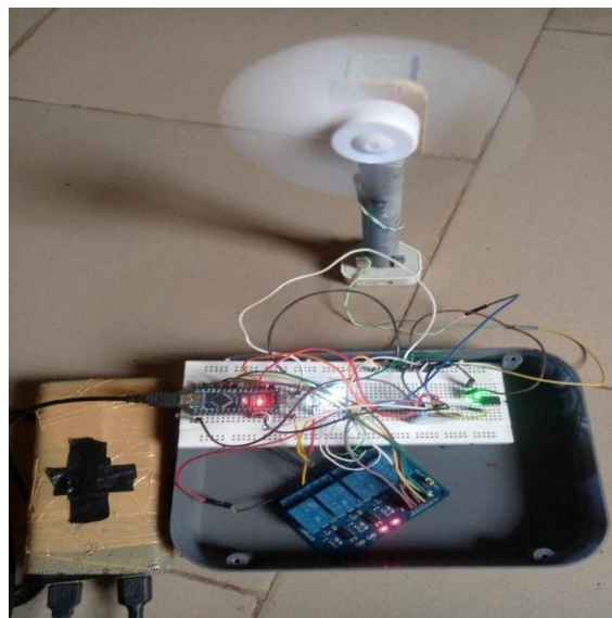
Figure 9: Prototype Implementation and Testing of the Circuit with a Mini DC Fan.
