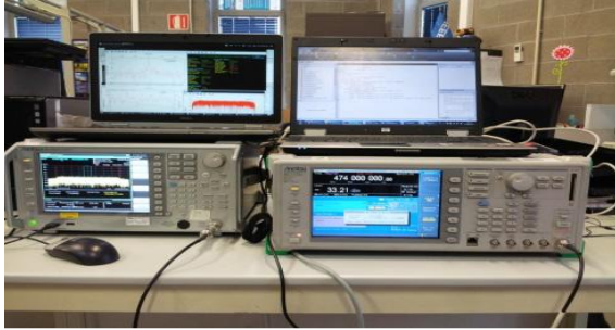
Figure 3.2: Equipment for monitoring digital penetration in the control centre
