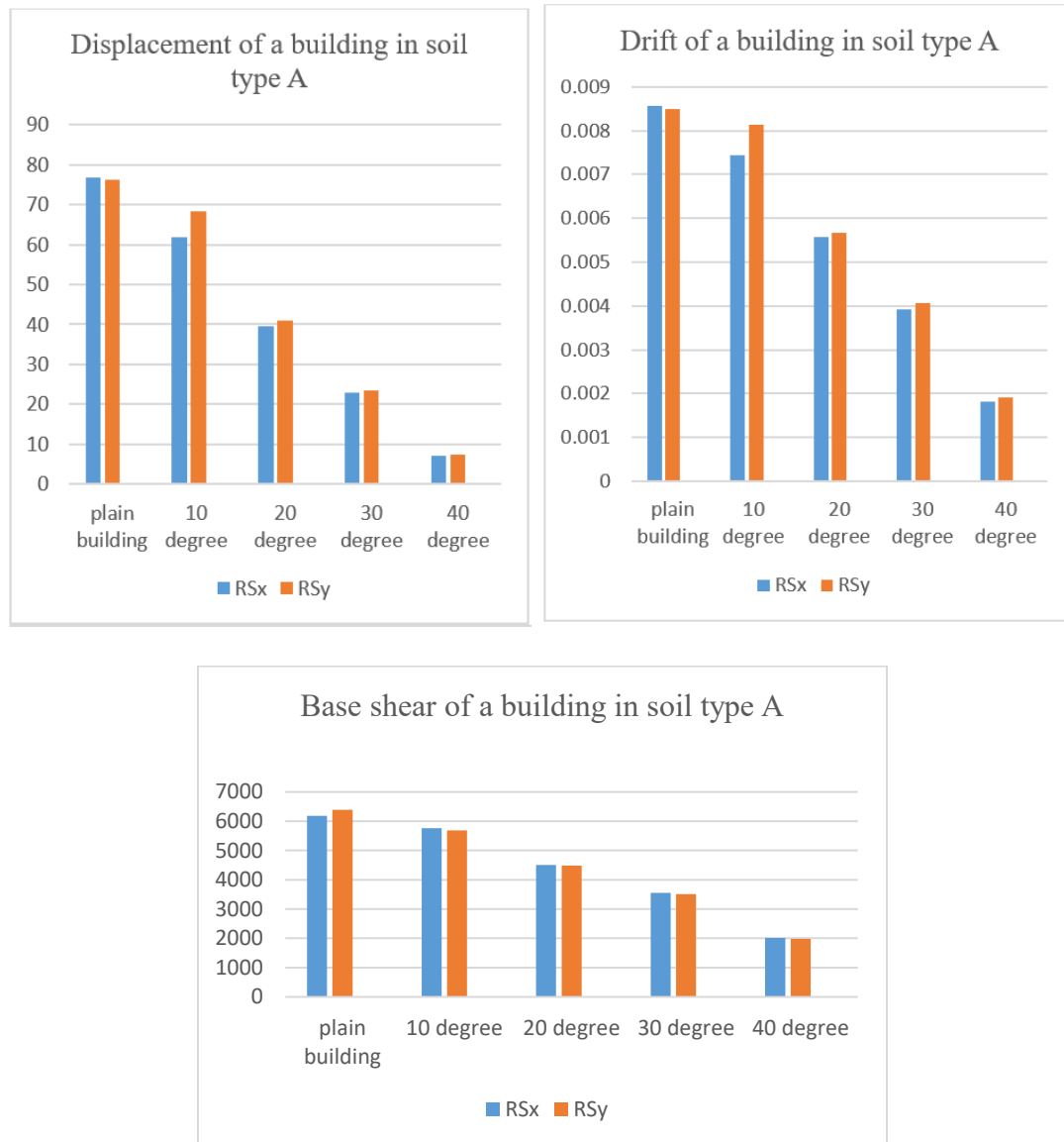
Figure 6: Comparison of story displacement, drift and base shear for a building in soil type A for EQX and EQY.
