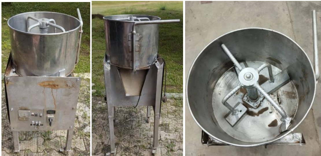
Figure 4: The finished foundry sand mixer
