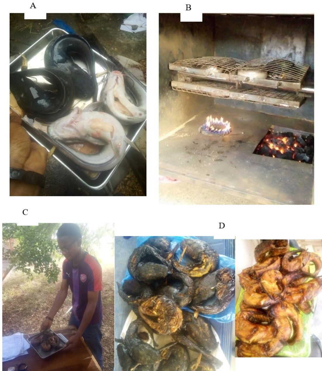
Plate 1: Performance Test with Full Cage-Tray Load; (a) Degutted and Curved Catfish (b) Inside the Dryer with Cage-Tray Load (c) Taking Dried Fish Moisture Content (d) Safe Dried Product to 15% db
