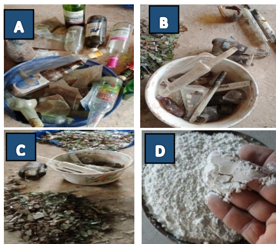
Plate 1 Samples of glass wastes used for this study. (A) Wastes alcoholic beverage bottles. (B) Wastes laboratory glass wares. (C) Wastes glass after pan milling. (D) Powdered glass wastes (GW) after ball milling
