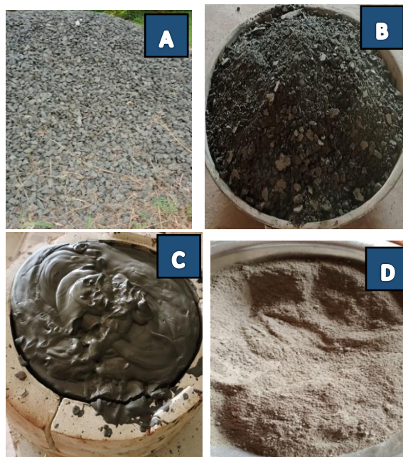
Plate 2 Samples of nepheline syenite (NS) used for this study. (A) Hip of NS supplied. (B) Crushed NS from panmill. (C) Dewatered milled NS from ball mill using POP mould. (D) Powdered NS obtained
