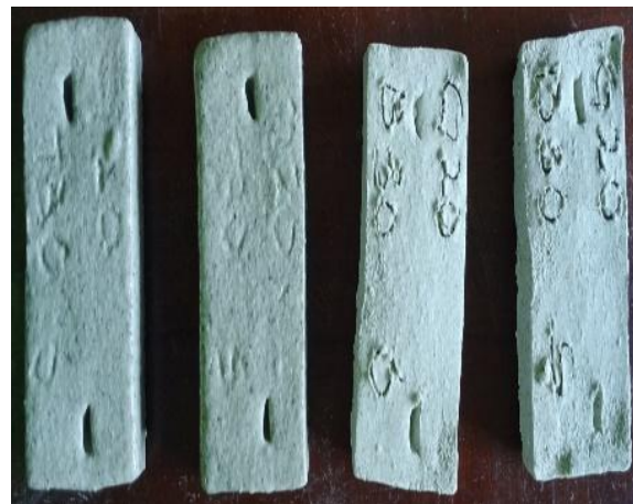
Plate 4 Comparative view of 30 % and 20% glass waste reinforced wall linings.
