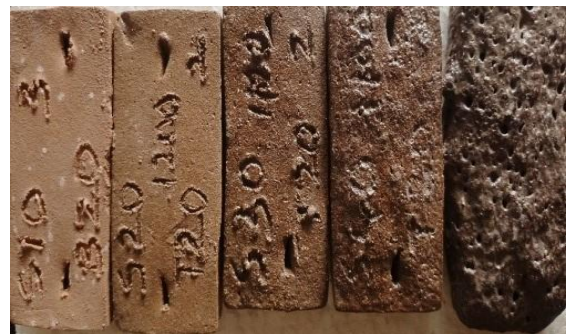
Plate 3 face valuation of nepheline syenite samples at different ratios for NS showing pinholes.
