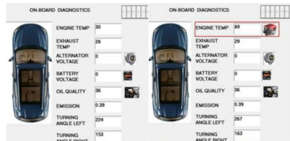
Fig. 4. Result of Temperature Sensor
