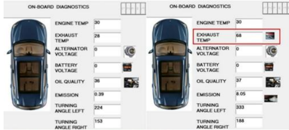
Fig. 5. Result of exhaust gas temperature sensor
