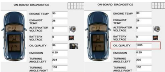
Fig. 7. Result of Oil level sensor
