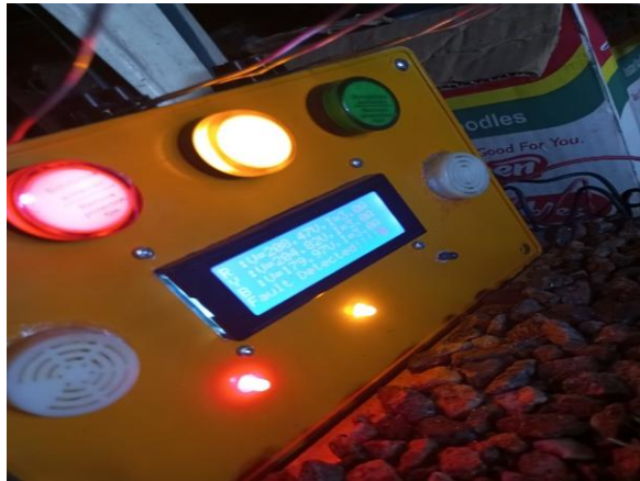
Figure IV-4 Diagram showing the switched of pilot light and relay indicator LED of the blue phase
