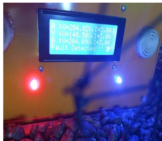
Figure IV-2 Diagram showing the switched off LED of the yellow Phase and the Voltage values in the system
