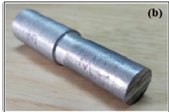
Figure 2. (a) Pin-on-Disc testing machine and (b) wear testing Pin
