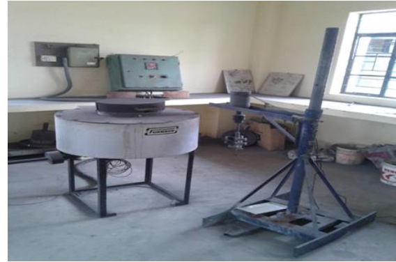
Figure 1. Electrical melting furnace and stir casting set up
