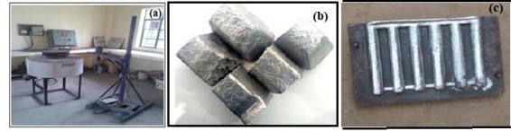
Figure1. Electrical melting furnace with stir cast setup, (b) LM13 ingot and (c) cast composite
