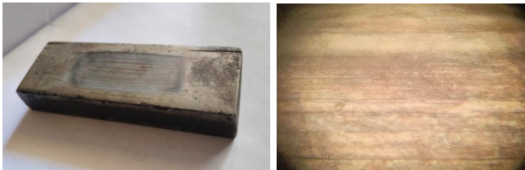
Figure4. Abrasive worn-out surface of MS at 12kg, 10min and 200 rpm
