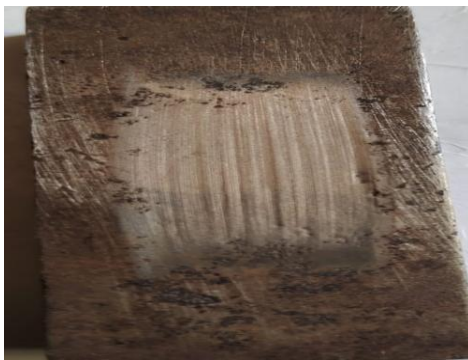
Figure3. Abrasive worn-out surface of MS at 12kg, 5min and 200 rpm
