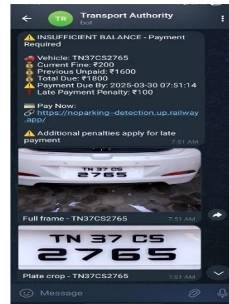
Fig no 4.1: Number plate detection & fine notification
