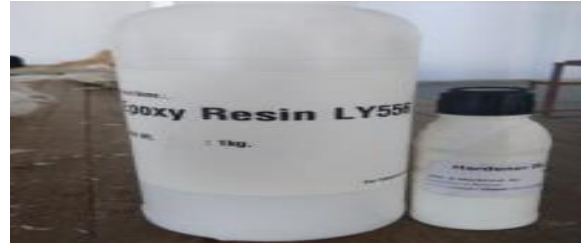
Figure 2.6: Epoxy (LY 556) And Hardener (HY951)
