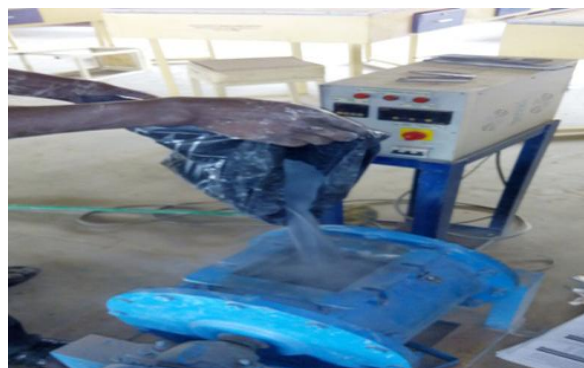
Figure 3: Ball milling using drum ball miller
