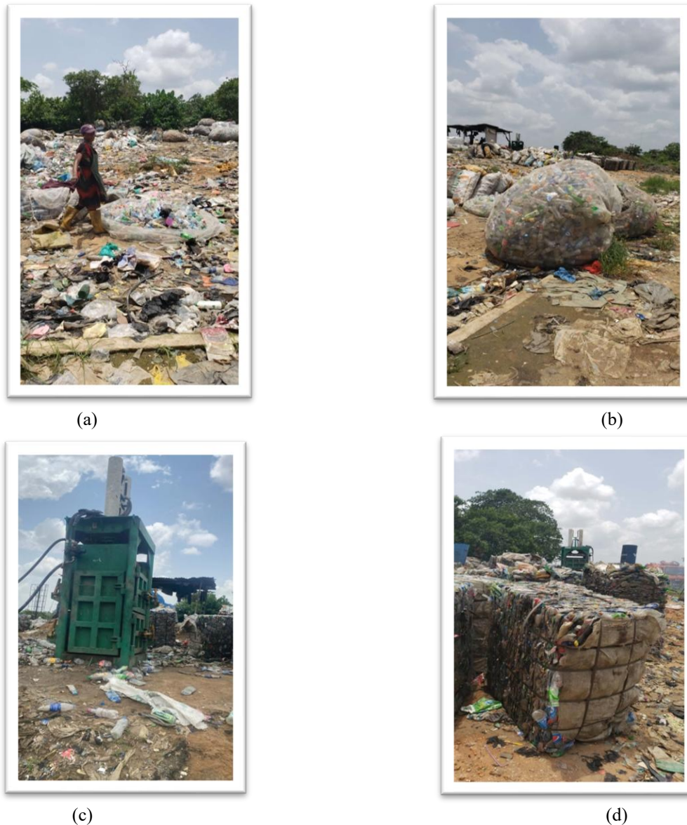
Fig. 4 (a) Manual sorting of wastes. (b) packaged sorted plastic wastes. (c) Compression machine (d) compressed and packaged wastes ready to be transported to recycling companies.
