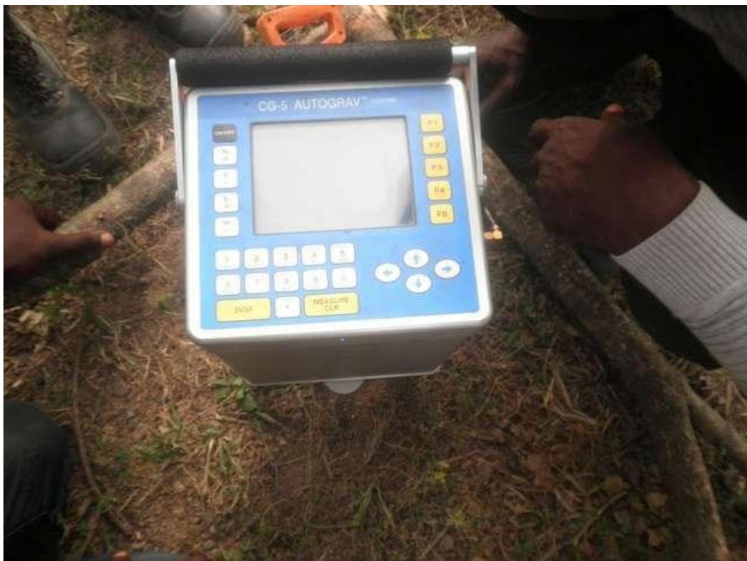
Figure 3.04. CG5 Autograv gravimeter used for the gravity data acquisition
