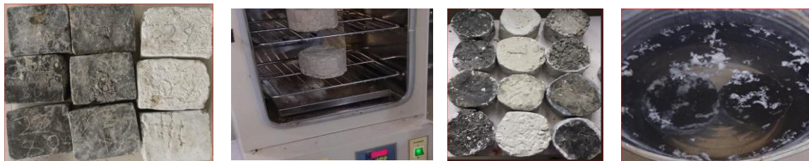
Plate 1: Compressive strength and sorptivity tests of concrete pave stone made from WPWS
