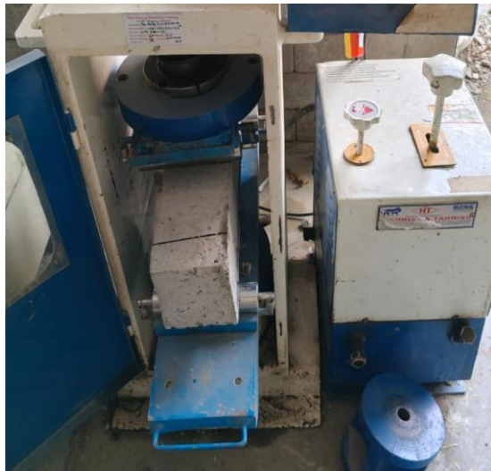
Figure 4. 2: Arrangement of flexural strength test Machine of beam in Lab
