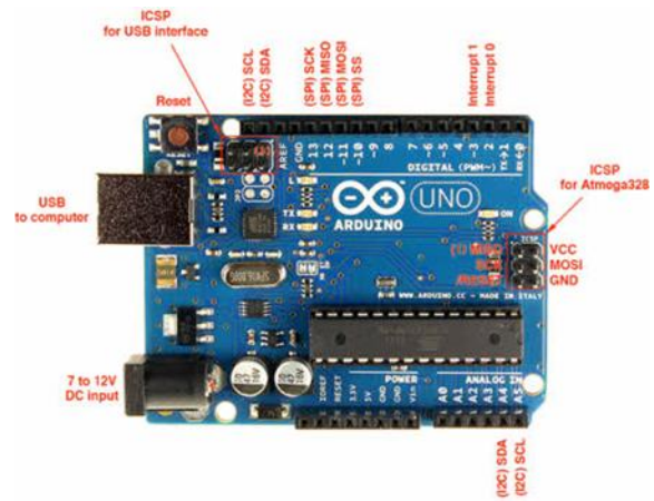
Fig. 1. Structure and parts of Arduino Uno
