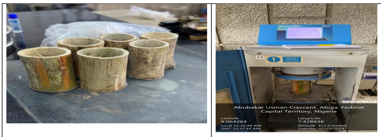
Plate 3.5: Compressive strength test specimens and set up
