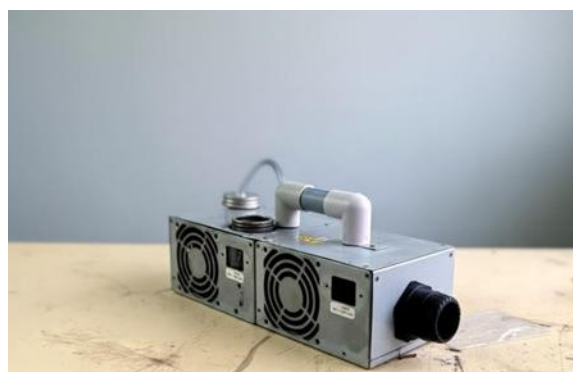
Fig.6: Developed Induction-Based Natural Repellent Vaporization System for Livestock Insect Protection
