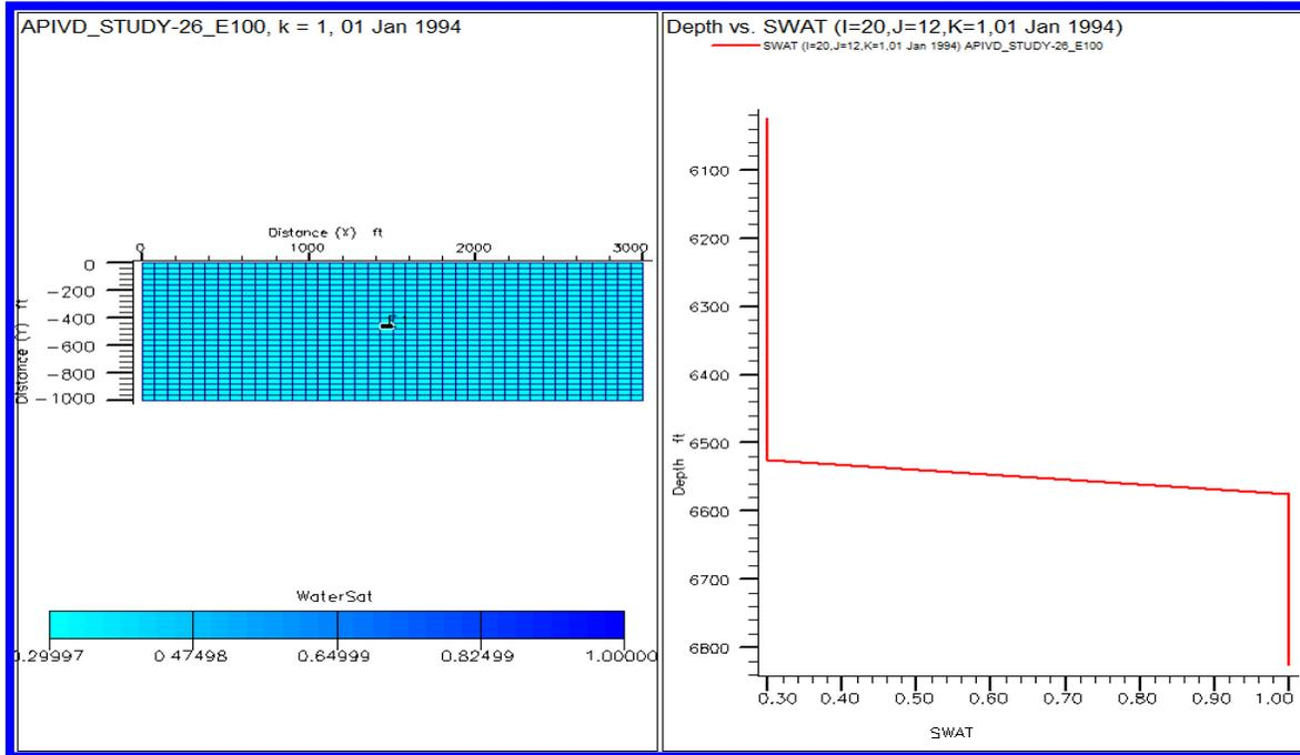
Figure 5.3: Initial water saturation distribution of the reservoir against depth
