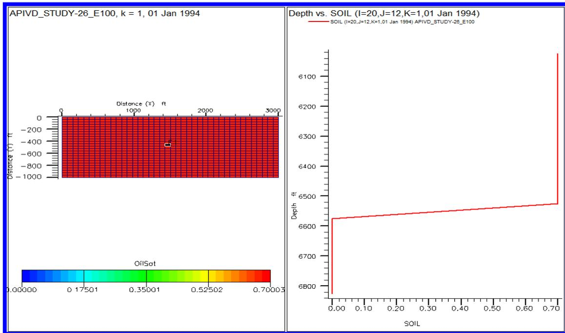
Figure 5.2: Initial oil saturation distribution of the reservoir against depth
