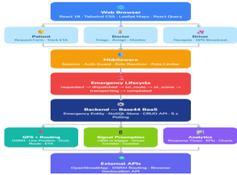
Fig 2.0: High-Level System Architecture
