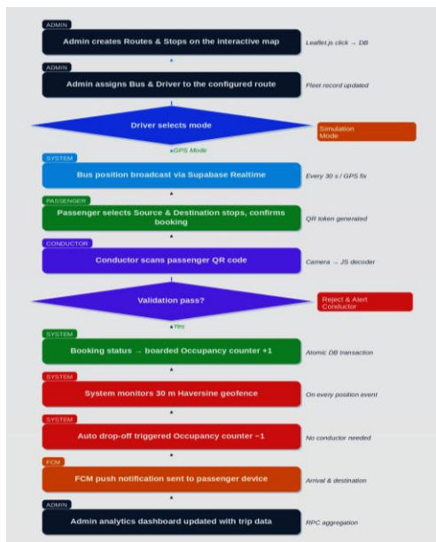
Fig. 5.1. End-to-end system workflow from Admin route configuration through automatic passenger drop-off and analytics dashboard update.
