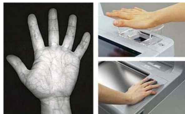
Figure 2.5 Hand palm vein scanning technique (Ruiz-Blondet, 2014)
