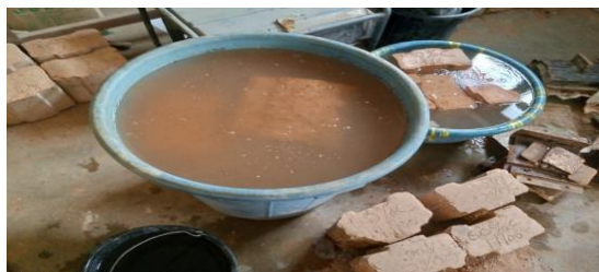
Plate 4c: Immersion of LIB in MgSO 4 Water Solution
