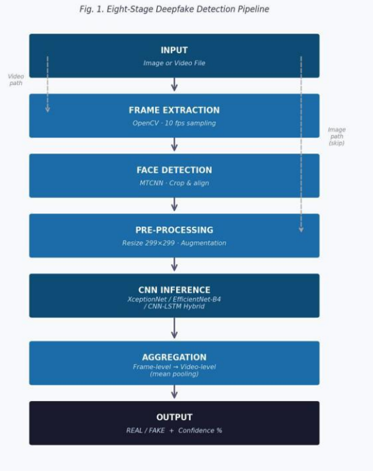
Fig. 1. Eight-stage deepfake detection pipeline from input ingestion through CNN inference to final verdict output
