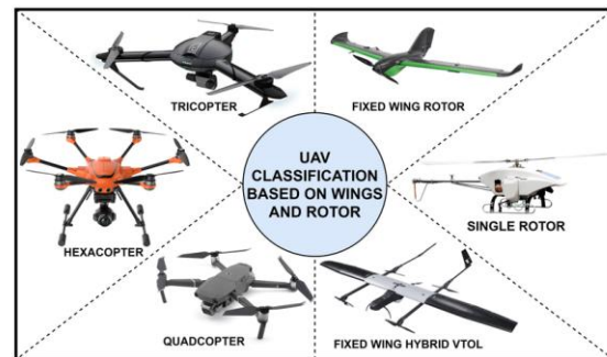
Figure 2: Classification of UAV based on wings and rotors (Chamola, et al., 2020).
