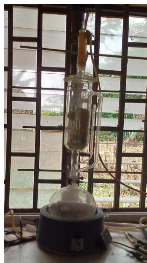
Figure 1: Extraction of rubber seed oil using Soxhlet apparatuses
