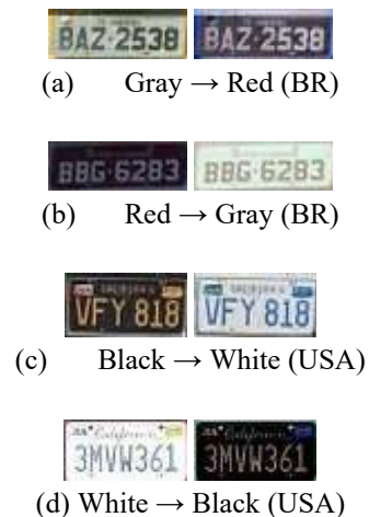
Fig. 4. Examples of negative images created to simulate LPs of other layouts. In Brazil, private vehicles have gray LPs, while buses, taxis and other transportation vehicles have red LPs. In the United
