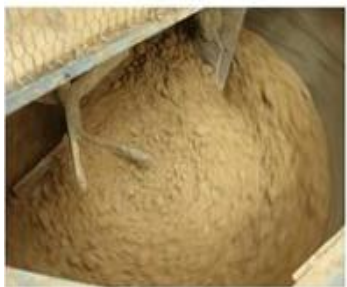
Plate 3: Dry Mixing of Materials
