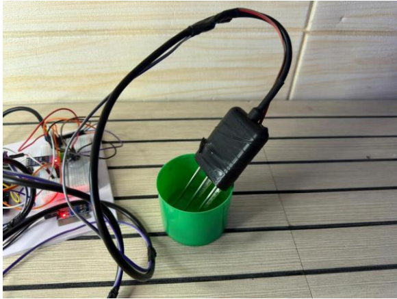
Fig. 2: NPK sensor probe inserted into soil sample contained in a field test vessel, demonstrating the probe insertion geometry during calibration verification.
