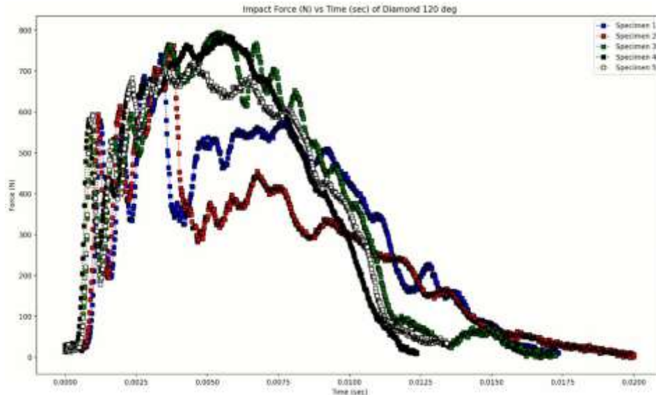
Figure 12. Impact Force (N) vs. Time (s) for the five 120° diamond sandwich panels, showing substantially lower peak loads (~760 N on average) and a broader time profile compared to the 45° diamond, indicating superior impact energy absorption.
