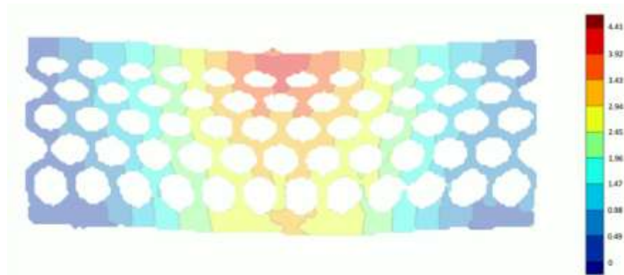
Figure 13. DIC y-axis displacement map (mm) for a functionally graded honeycomb specimen under 3-point bending, showing the displacement gradient from the loading nose contact point (red, ~4.41 mm) to the support regions (blue, ~0 mm).
