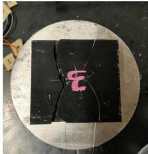
Figure 6. Post-impact specimen showing the characteristic fracture pattern at the impact point centre, with crack propagation to the face sheet.
