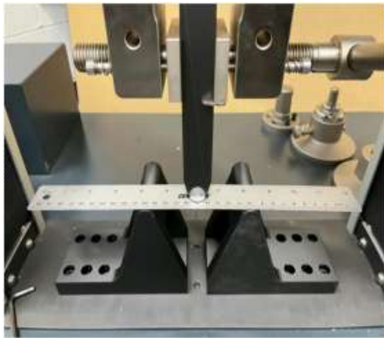
Figure 5. Three-point bending test setup showing the loading nose and two support points with 100 mm span.
