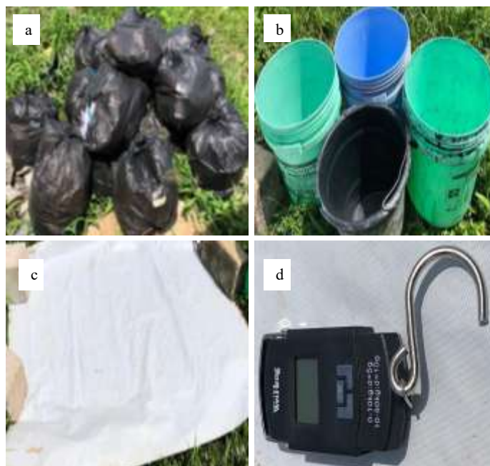
Fig. 3: Waste collection and separation process (a) Samples of waste collected and separated, (b) Sorting containers, (c) Sorting platforms and (d) Digital hanging weighing scale.
