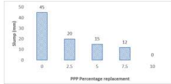
Fig. 7. Slump value against percentage of sand replacement with polypropylene in concrete
