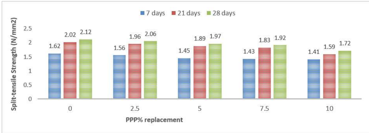
Fig. 10. Split-tensile strength of concrete mix with increasing concentrations of PPP during various curing days.
