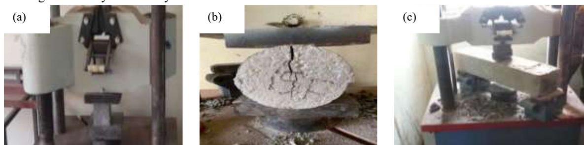
Fig. 5. The mechanical test includes (a). Hardened cube concrete tested by a Universal testing machine, (b) Hardened cylindrical concrete tested by a Universal testing machine, and (c) Hardened reinforced concrete beam tested by a Universal testing machine
