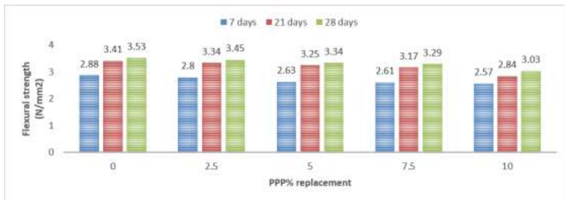
Fig. 11. Flexural strength of concrete mix with increasing percentages of PPP during various curing days.
