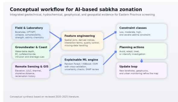
Figure 1. Apple-inspired conceptual workflow linking geotechnical, hydrochemical, geophysical, and geospatial evidence to explainable machine-learning zonation outputs.
