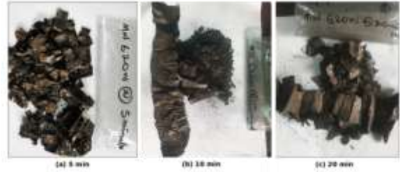
Figure 3: Representative morphology of electrode materials treated at 620 W for 5, 10 and 20 min
