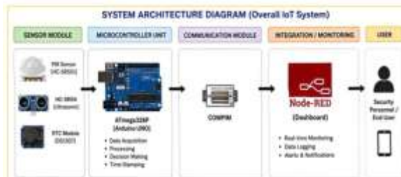
Fig. 1. Proposed Adaptive IoT-Based Surveillance System Architecture
