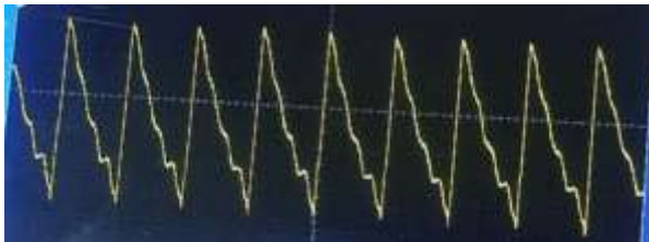
Figure 9: Pulsating Excitation Voltage 300 Hz
