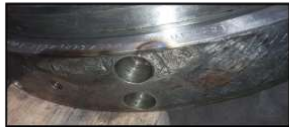
Figure 6: Discharge evidence at torus contact surface.
