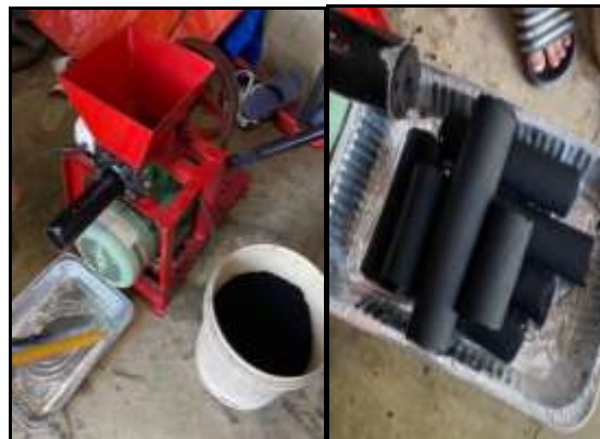
Fig. 1. Briquetting of torrefied biomass
