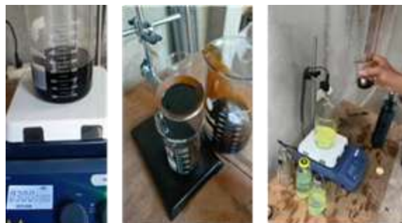
Figure 1. Purification process of the tire pyrolytic oil and blending with diesel: (a) heat treatment, (b) filtration, (c) blending with diesel
