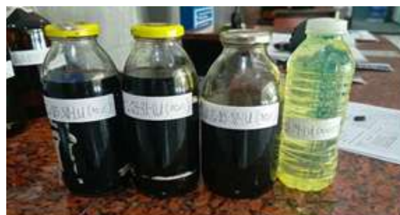
Figure 2. 10%, 20%, 30 Blends of Tire Pyrolytic Oil-Diesel Fuel for Testing
